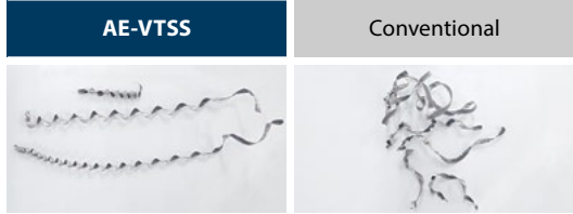
Chip shape from plunging
